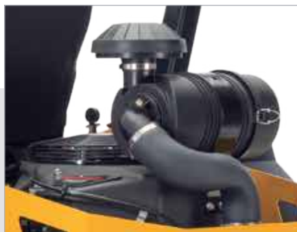
KAWASAKI ® FX ENGINE With multi-stage canister air filter
