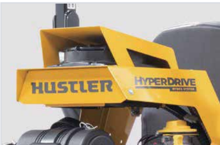
9 in. Fan & High-Capacity Oil Cooler with Hot Oil Shuttle
